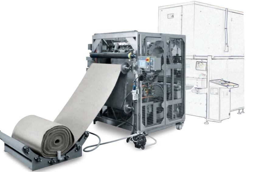
*The FOAMLINER provides the ultimate precision in foam impregnation by means of direct pressurised injection of foamed reactive resins or blenders into natural fibre mats. Ideal fields of operation for the FOAMLINER are the manufacture of door lining in automotive industries or applications in textile industries.*
